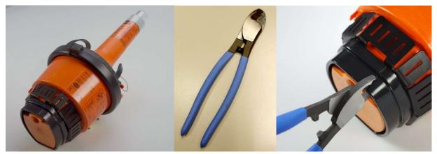
Tron 40VDR with storage module ready for removal
