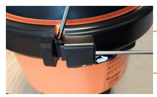
Then take another screwdriver and pry the two halves of the Equator Belt apart.
