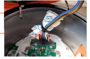
Snip off the battery connection cable close to the circuit board. This renders the electronics unusable.
