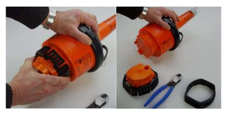
Take a solid grip around the Storage Module and release the unit from the Capsule
