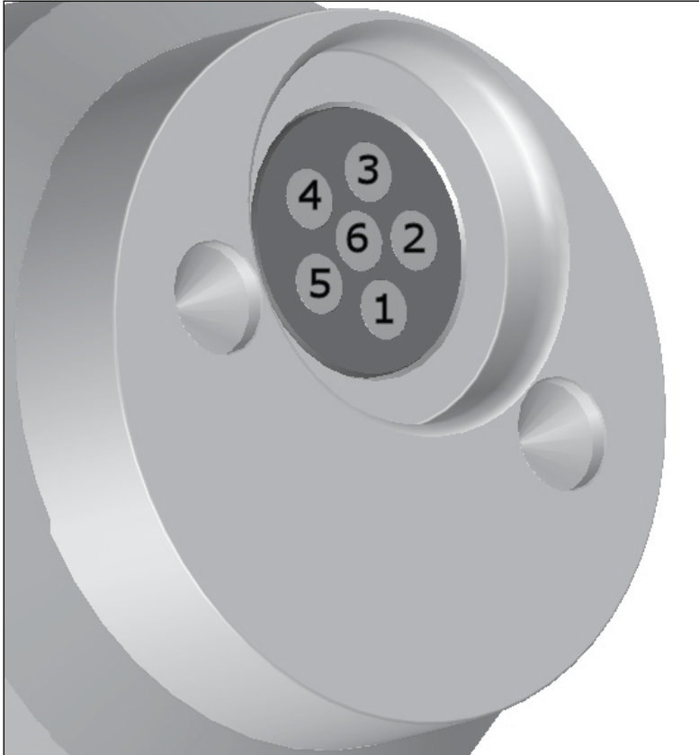
Figure 3.1.6.1, S-VDR female connector in capsule.
