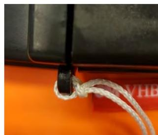
6. Remove protecting paper from double-sided tape, MAKE SURE THE RED PART OF WRIST STRAP DO NOT COVER LABEL and press the wrist strap in place.
