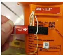
6. Remove protecting paper from double-sided tape, and press the wrist strap in place. Keep the pressure for 10 seconds with two fingers along the red tape wrapped around the wrist strap to ensure good bonding..
