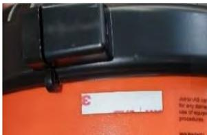
Keep the pressure for 10 seconds with two fingers along double-sided tape to ensure good bonding to the EPIRB.
