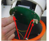
Disconnect Battery, Water switch and FRM (Final Recording Medium) connectors
