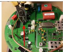
Dissassemble all PCB's and cut off uProcessor crystal as seen here. (Makes the electronics unusable)
