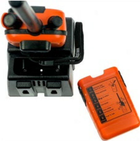
Figure 7 Tron TR30 radio in the charging bay
