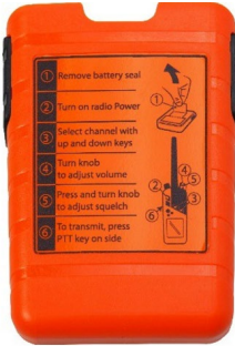
Figure 4 Tron TR30 Emergency battery (orange)
