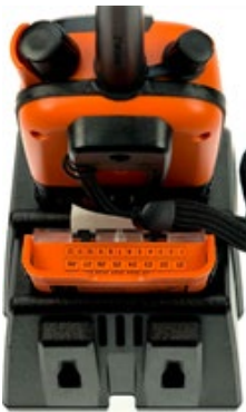
Figure 8 Emergency battery in the storage bay
