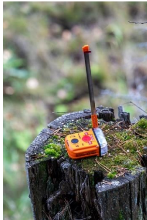
Place the PLB on a flat surface
